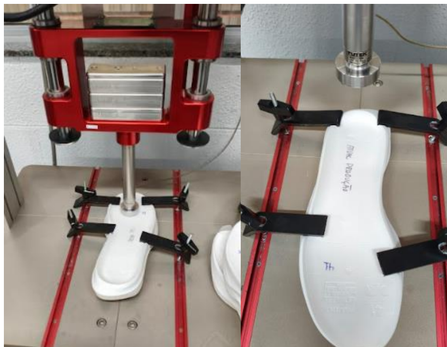
Figure 3. Equipment for measuring energy loss, force apply in rearfoot and forefoot.
