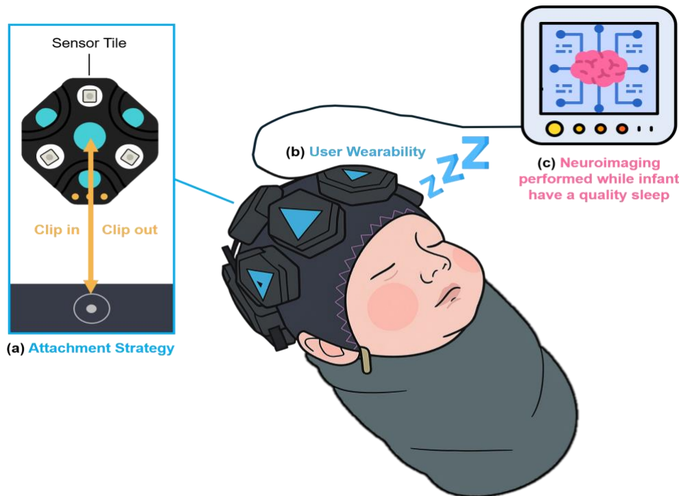
Figure 6. Uchitel et al.'s device function wearability and modular attachment strategy. (a) The sensor tile is built with a clip mechanism that can fit into specific parts of the cap. (b) Each sensor tile can be positioned in different parts of the cap, enabling adaptability for multiple head shapes. (c) The cap platform is thought to be a comfort resource, so that brain activity supervision and imaging can be performed while the baby is deep asleep. Illustration created with the assistance of artificial intelligence. This image is merely illustrative and is not included in, nor part of, the article on which it is based
